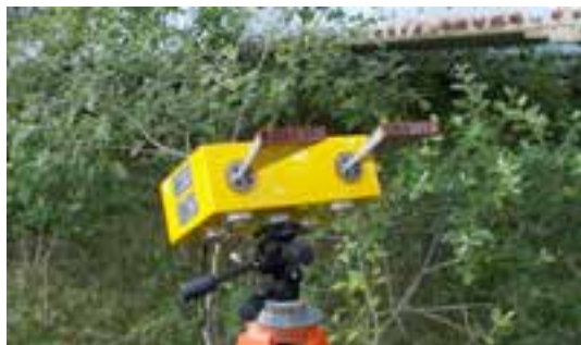
Obr. 1: Interferometrický radar IBIS-S
